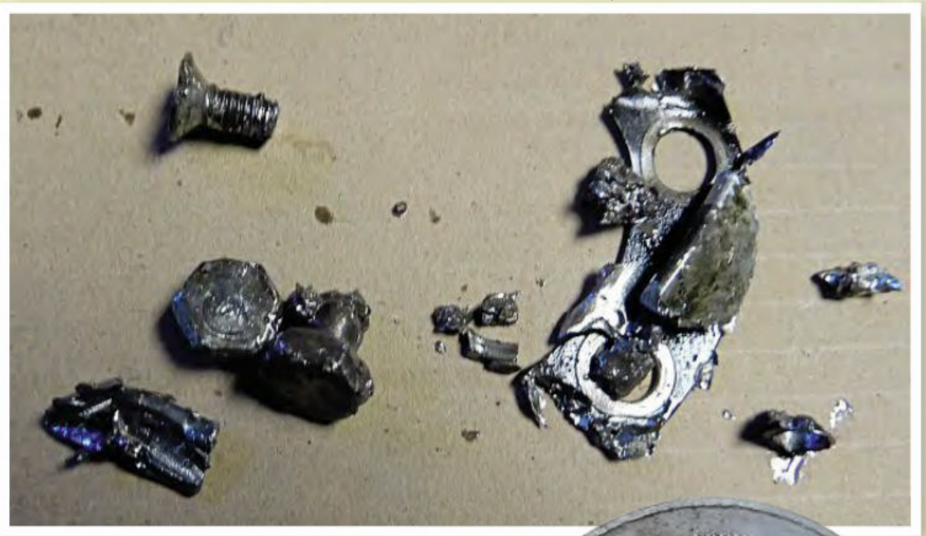
Above and right: Bolts retained by tab washers rarely break loose. When they do, the results can be fairly scary
