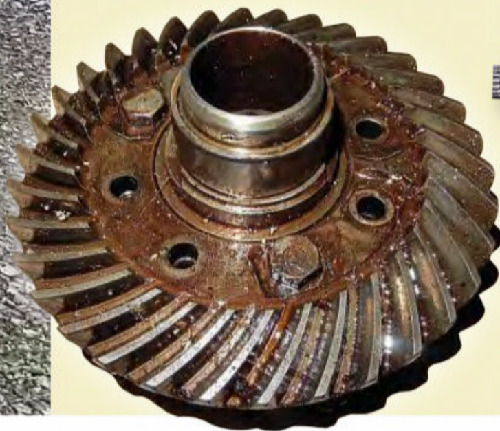
Above and right: Bolts retained by tab washers rarely break loose. When they do, the results can be fairly scary
