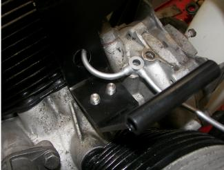
Step Eight: Place supplied Alternator into bracket. Belt can be placed over pulley at this point also. Using the bolt on the right side of the bracket thread into the Alternator mount ear, do not fully tighten. Place M10 bolt into left side of bracket from rear.
